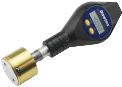
SmartPlug with TiN coated body
