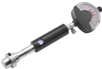
SmartPlug with depth stop
